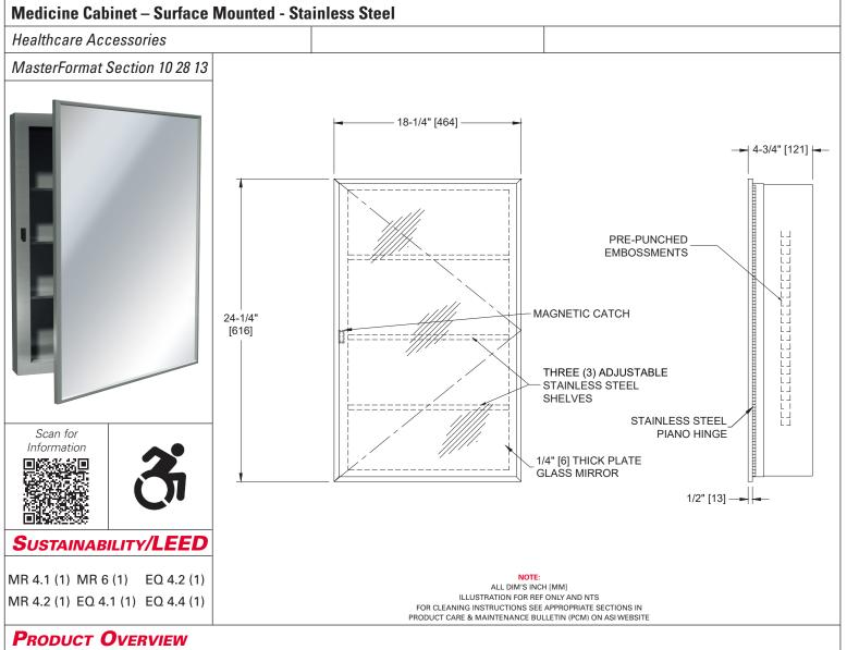
Surface mounted cabinet. Mirrored door is hung on cabinet with a full length 3/16" [04,7] heavy duty stainless steel multi-staked piano hinge. Cabinet has three adjustable stainless steel shelves. Access is gained to the three (3) adjustable shelves by disengaging magnetic catch and swinging open the door. Adjustable shelves permit storing various size articles.
