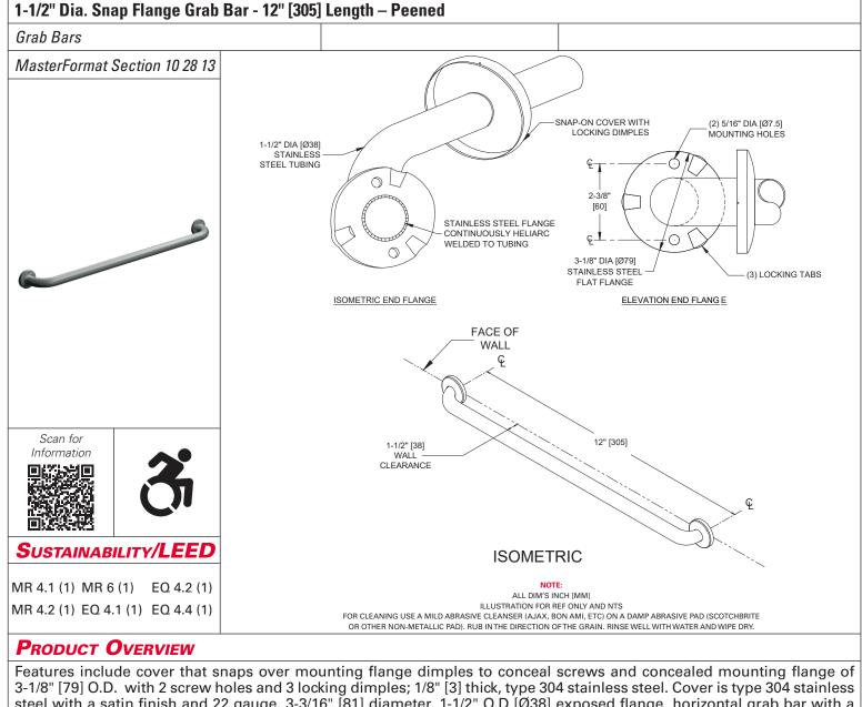
steel with a satin finish and 22 gauge, 3-3/16" [81] diameter. 1-1/2" O.D [Ø38] exposed flange horizontal grab bar with a peened surface.
