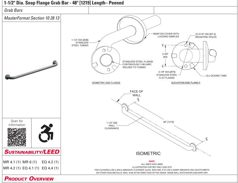
Features include cover that snaps over mounting flange dimples to conceal screws and concealed mounting flange of 3-1/8" [79] O.D. with 2 screw holes and 3 locking dimples; 1/8" [3] thick, type 304 stainless steel. Cover is type 304 stainless steel with a satin finish and 22 gauge, 3-3/16" [81] diameter. 1-1/2" O.D [Ø38] exposed flange horizontal grab bar with a peened surface.
