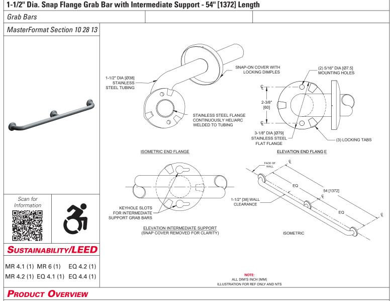
Features include cover that snaps over mounting flange dimples to conceal screws and concealed mounting flange of 3-1/8" [79] O.D. with 2 screw holes and 3 locking dimples; 1/8" [3] thick, type 304 stainless steel. Cover is type 304 stainless steel with a satin finish and 22 gauge, 3-3/16" [81] diameter. 1-1/2" O.D [Ø38] exposed flange horizontal grab bar with a smooth surface.
