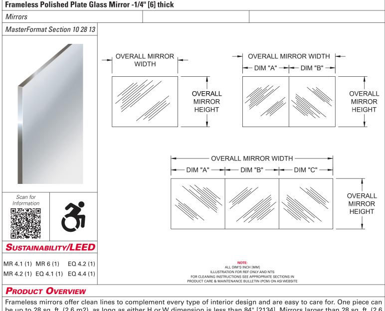
be up to 28 sq. ft. (2.6 m2), as long as either H or W dimension is less than 84" [2134]. Mirrors larger than 28 sq. ft. (2.6 m2) or with either linear H or W dimension larger than 84" [2134] shall be supplied as multiple pieces. Made of 1/4" [6] polished plate glass.
