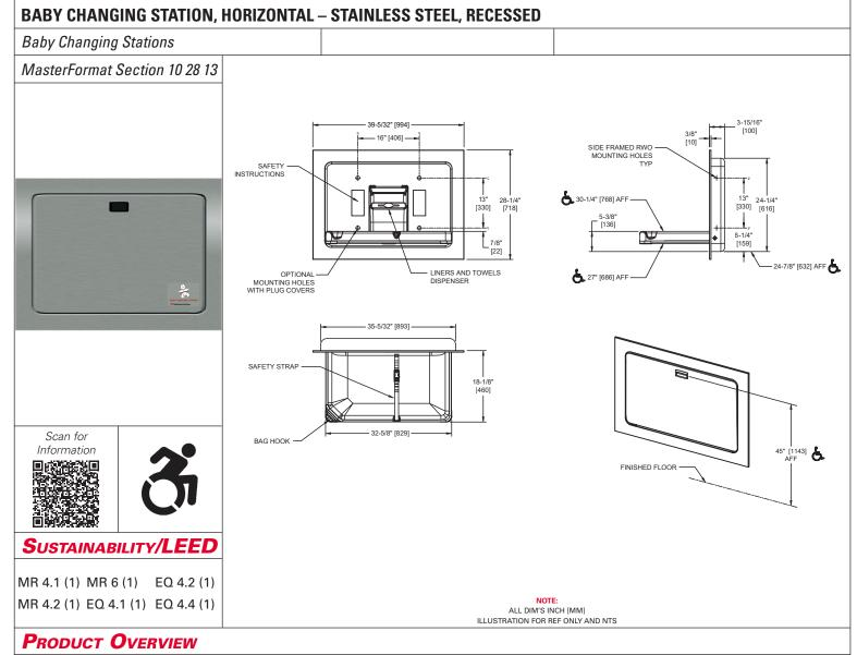
This horizontal station has a door facing and collar made from 20 gauge 304 stainless steel. Fabricated of FDA-approved fungus and bacteria-resistant plastic. Unit complies with 2010 ADA Accessibility Standards and supports a static load of 300 lbs. (136 kg) and be tested in excess of 350 lbs (159 kg).
